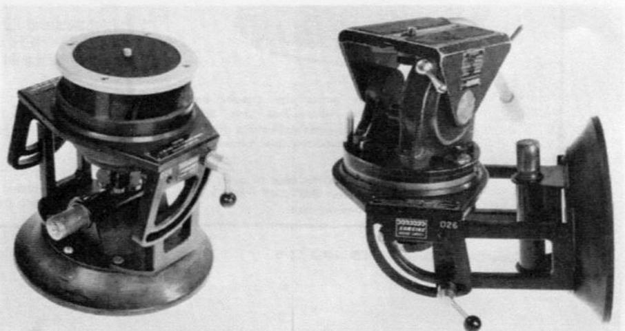
(LEFT) Samcine Super Limpet Mount in horizontal position with flat-top adaptor fitted. (RIGHT) Super Limpet Mount in vertical position with a pan and tilt head fitted. The Limpet is a mount with tremendous holding power for mounting cameras to flat or curved surfaces of vehicles, and is adaptable to a number of other applications.
