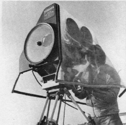
The Samcine Rain Deflector is handy for filming storms at sea. The whirling glass disk in front of the lens keeps the field free of water spray.
