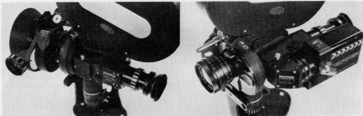
(LEFT) Arriflex 2C with Samcine Follow-focus Matte-box and Samcine "Italian" Door. (RIGHT) Samcine "Italian Door" and Samcinevision TV Viewfinder. Samcinevision was first used by Oswald Morris, BSC, for photographing OLIVER in 1967. Samcinevision has been in constant development ever since. Nowadays Samuelson's has models to fit almost any 35mm film camera, available in color, as well as black and white.
