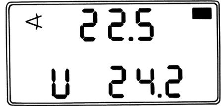
LCD display with PHASE button pressed. Open mirror shutter angle (22.5°) and battery voltage (24.2 V) are visible.
