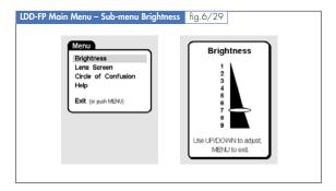
By briefly pushing the SET button, the Brightness Screen will appear. By using the UP and DOWN buttons, the brightness can be adjusted. When leaving the Submenu, the new adjustment will be saved.
