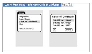
After having selected the Sub-menu circle of confusion, the coc screen will offer three options. To select the appropriate option, move the cursor on it and push the SET button. Then move the cursor to **Done** and press SET to return to the Main Menu. When pushing the MENU button for 3 sec. the Lens Screen will appear.
