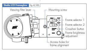
By means of a sophisticated electronic design, the Studio LCD Frameglow fades in one or – simultaneously – two luminous frames. Four frame outlines with the following aspect ratios are provided in the Studio LCD Frameglow:
