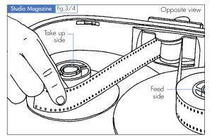
10. Attach to take up core. Feed film into core slot so that no acute angle forms when turning the core clockwise. Wind just enough film around take up core to make sure it will not accidentally slide out again. Wound up film has to be flush with the core and lie flat on take up plate or coreholder disk.
