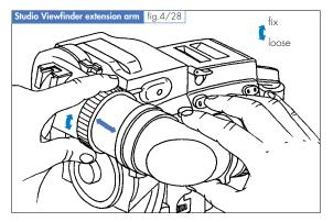
The other end of the Viewfinder Arm provides a mini PL bayonet mount to attach the Eyepiece. In order to adjust the Eyepiece position for a comfortable viewing, loose the eyepiece rotation friction knob located on the bottom side of the Viewfinder Arm.
