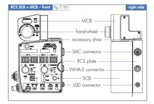
Because the SAC connector of the RCS is similar to the ones of the SCB and the MCB Cable Adapter, the same cables can be used for connecting the Remote Control Station with the camera.
