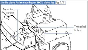
After removing the protection cover (two 3 mm hex screws) and checking that both parts (connectors, glass surfaces) are absolutely free of dust and fingerprints, mount the Video Assist to the Viewfinder or 100% Video Top. While tightening the screws, the connectors will fit together automatically. Therefore be sure that the Video Assist sits securely on the Viewfinder or Video Top.
