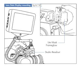
A Backplate together with the Shoe Post allows the LDD-FP Holder to be mounted on any Accessory shoe. A collapsible Sunshade attaches by means of Velcro.
