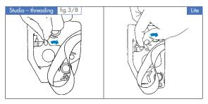
4. Pull some film out of the magazine until the loop is about one hand width long.
