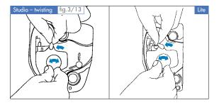
To adjust loop length, turn INCHING knob to the position (dot) labelled "LOOP".
