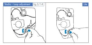
10. Form upper film loop by depressing and turning the sprocket roller. It should follow the "LOOP" mark engraved on the rear of the camera interior.
