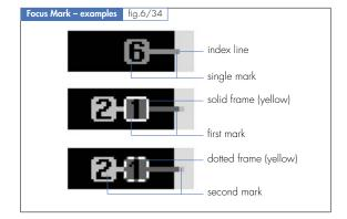
The Display's Focus Marks are square; a number and a colour will automatically be assigned. If a Focus Mark must be identified for moving or renumbering purposes, a solid or dotted yellow frame will surround this selected Mark.
