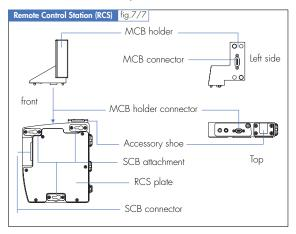
On top of the RCS Plate, a fixture for the MCB Holder as well as an Accessory Shoe is located. After removing the little cover on top of the RCS, the MCB Holder can be fixed with one 3 mm hex screw. The MCB will be mounted on the Holder in the same way it is fixed to the camera.
