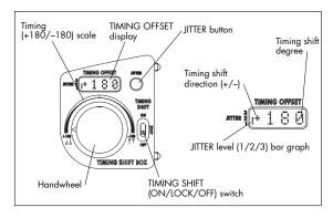
The Timing Shift Box (TSB), allows the creation of a streaking effect by manually adjusting the phase relationship of the mirror shutter to the movement. The timing shift effect can be adjusted from very faint to very strong.
