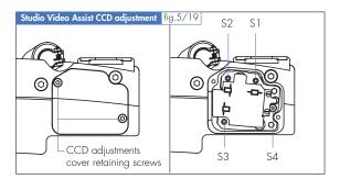
Three screws allow the fine positioning of the CCD and one screw (S4) moves it in and out to obtain the best possible focus.
