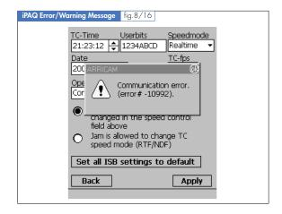
If a Sub-menu is active (the ERRORS/WARNINGS Info Box excepted) and the communication is lost, an Error/ Warning Message appears and the program returns to the Main Menu.
