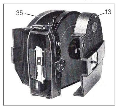
When using raw stock on plastic cores the film core holder (g) is put on the feed shaft, the film roll with the core is pushed onto the film core holder and secured by swinging the flap back and tightening it. Daylight loading spools are placed directly on the feed shaft and also secured.
