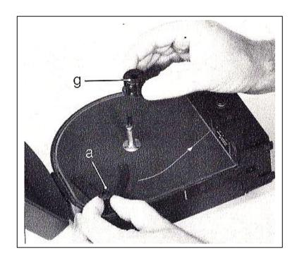
under the threading slot. Film run in direction of the arrow and the correct positioning of the perforations can only be obtained when "B winding" film is used as previously described.
