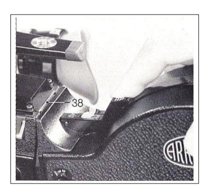
raising the magazine and removing it from the camera's snap catch (38).
