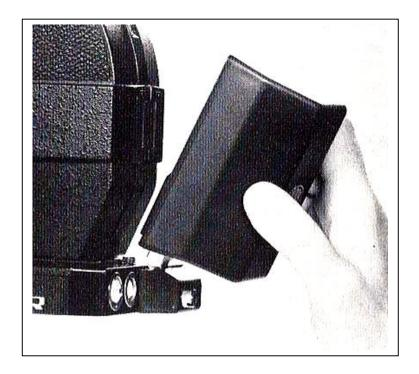
The camera can also be run from a 12 V battery connected with a power cable (mode) KCU). The 4-pole battery connecter and its cabling is identical to that used with the ARRIFLEX 16 BLEQ and the ARRIFLEX 35 BL. The camera battery is used to run the quartz controlled drive motor, the exposure meter and automatic diaphragm control as well as all the electrical accessories.
