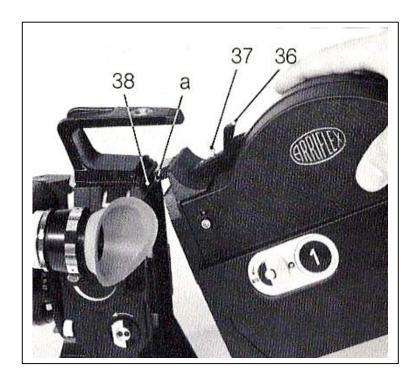
Finally, the magazine release catch (36) is locked by pushing back the lever (37) to "Lock"; the camera is then run a few turns slowly by pressing the test button (30) until the film transport claw engages with a perforation hole.
