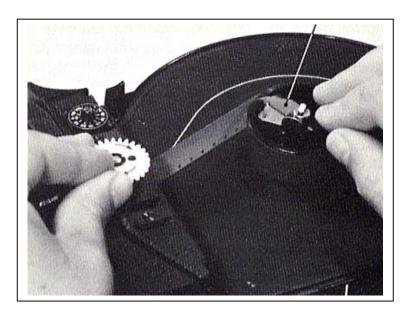
for using raw stock with plastic core, the pressure roller is not swung onto the spool but remains latched away from the spool. In this case the counter works only for the exposed film (12). 1t must be reset to "0" every time the film is changed.
