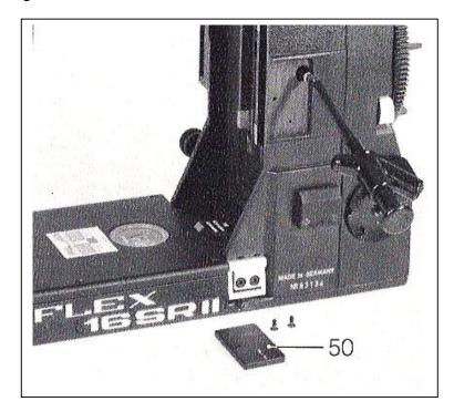
To replace the lamp, first remove both counter sunk screws. When the magazine is removed the cover plate (50) can be lightly pulled up so that the threads for the full frame start marking lamp are visible.
