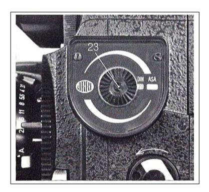
consideration during shooting as polaroid filters affect the light measuring. Regardless of the focal length of the lens used, in this exposure metering system about 25 % of the central image area is measured.
