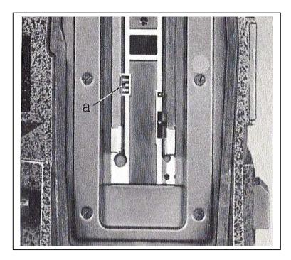
The film is exposed on the opposite side of the claw, two frames below the gate (a).
