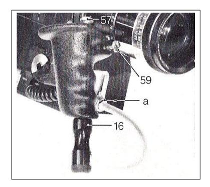
until resistance is felt. Finally, the protecting collar (16) is placed into the handgrip hole until it locks. To remove - follow steps in reverse order.
