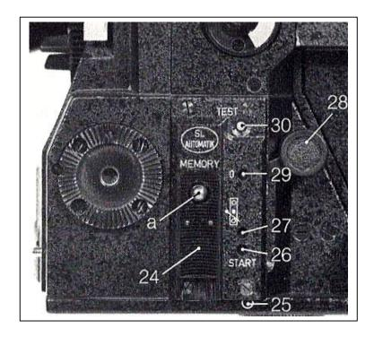
When the camera has been unused for a longer period of time or when it is cold, the inching system should be switched on for a short time to prevent damage to parts which have become sluggish. The inching system can be switched on by depressing the small red test button (30).
