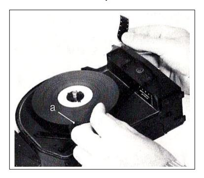
the magazine gear be turned by hand in the same direction (so that the film length remains unchanged) until the film head appears in the take-up area.
