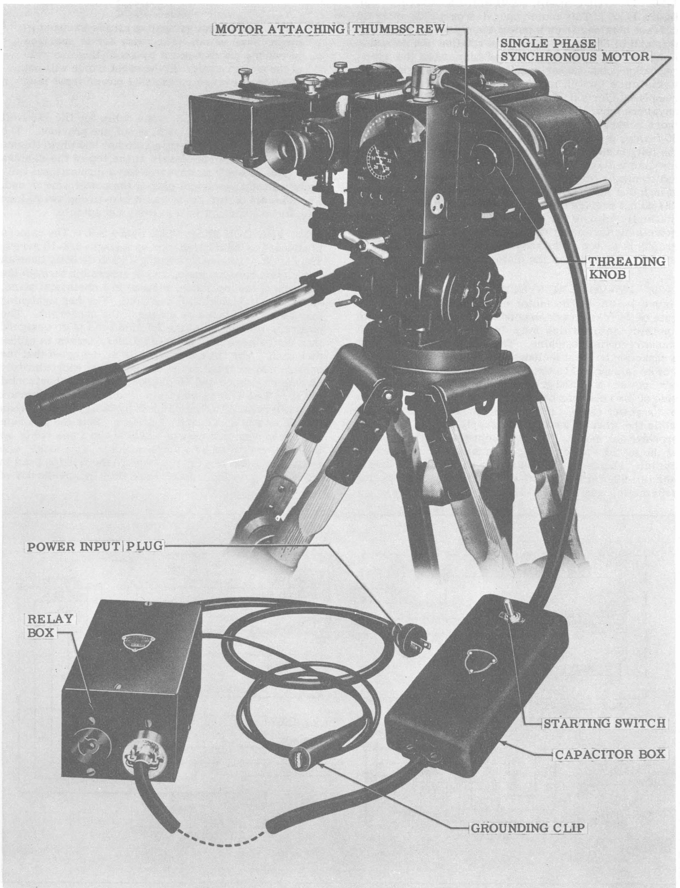
Figure 1-13A. Electrical Hook-up for 115 Volt Ac Synchronous Motor
