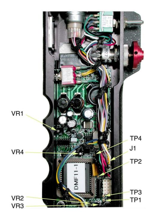
Fig.3 Circuit board showing test points and potentiometer locations.
