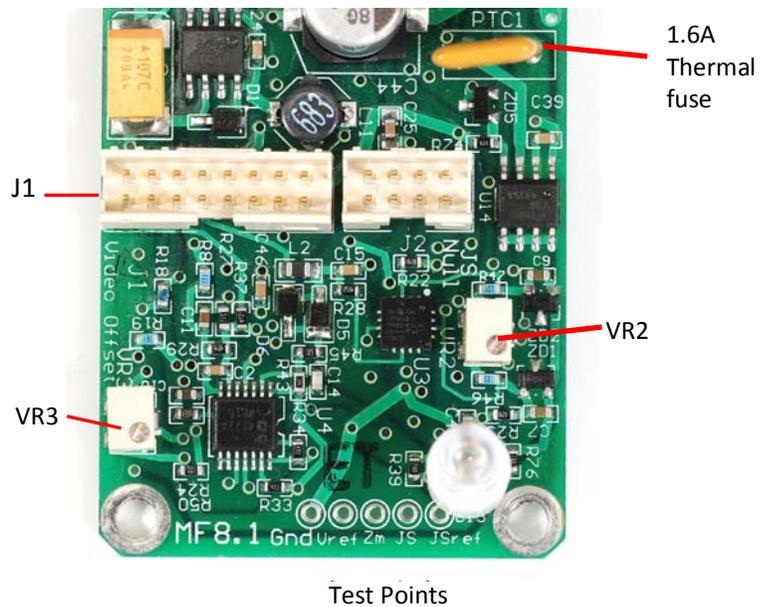
iv. J1 16-pin Berg Connector Pin Functions
