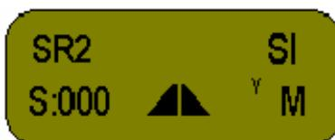
The top line on the display indicates the type of camera controlled (**SR11** in this case) and the program activated (speed/iris, **SI**).
