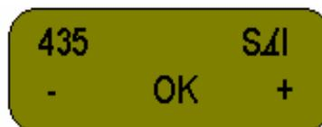
Trough the “+” and “-“ buttons, you can select the type of compensation program you would like to run. Once a program has been selected, press the **OK** button to activate the program and switch to the next screen.
