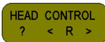
This program is intended so that the camera assistant who changes the magazine can control the head but the person at the central control unit cannot. This function is also useful in setting up future shots. With this program engaged, the control unit is completely overridden..
