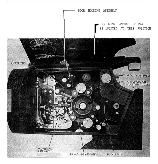
ATTACH DOOR HOLDING ASSEMBLY TO NEW VIDIFLEX 2.
