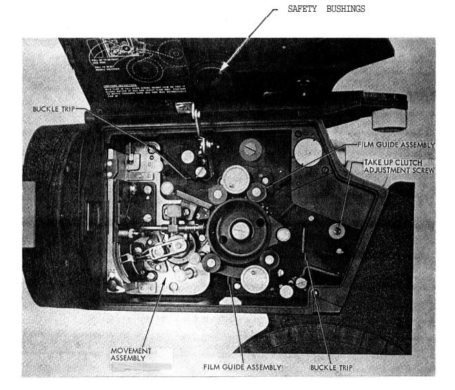
REMOVE THE MITCHELL DOOR FROM YOUR CAMERA AND INSTALL THE FILM KEEPER SAFETY BUSHINGS FROM THE ORIGINAL DOOR ONTO THE VIDIFLEX 2 DOOR.
