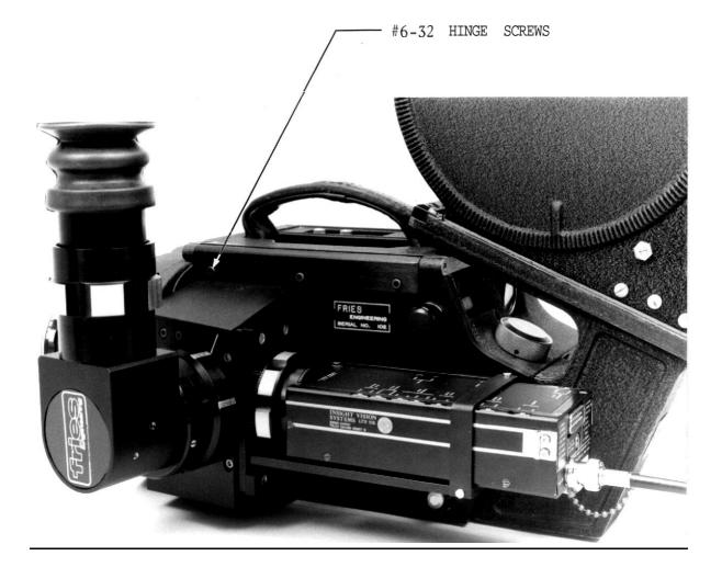
LOOSEN THE 3 #6-32 SCREWS ON THE HINGE AND FIT THE VIDIFLEX 2 DOOR ON THE CAMERA BODY. INSTALL BOTH HINGE PINS, THEN RETIGHTEN THE 3 HINGE SCREWS. OPEN AND CLOSE THE DOOR TO CHECK FOR PROPER FIT AND, IF NECESSARY, LOOSEN THE HINGE SCREWS AGAIN AND REALIGN THE DOOR TO THE CAMERA BODY BEFORE RETIGHTENING.
