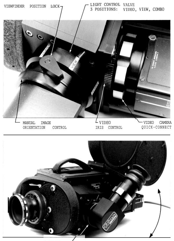
MANUAL IMAGE ORIENTATION CONTROL CAN BE USED TO CORRECT BEYOND THE 180° RANGE.
