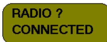
In the event that the channel selected on the hand unit does not correspond with the channel selected on the Motor Driver box; the system will stay blocked displaying the following screen until the channels are matched
