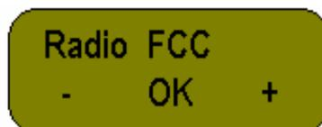
By pressing the “+” and “-“ buttons, one of the following standards can be selected: **FCC, IC, ETSI, SPAIN, FRANCE and MKK** (the number of channels for each standard depends on the regulations for each area). After the standard for the area you are operating the system in is on screen, press the top-center button to activate
