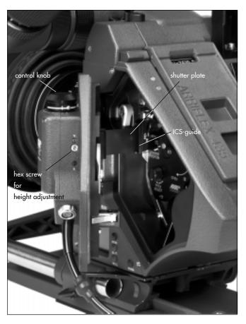
Press the control knob photo on the Integrated Capping Shutter and turn until the black plate reaches the ICS-Guide.
