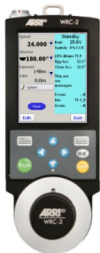
Wireless Remote Control WRC-2 K0.60042.0 includes: WRC-2 Main Unit, K2.65128.0 Control Knob Unit, K2.65129.0
