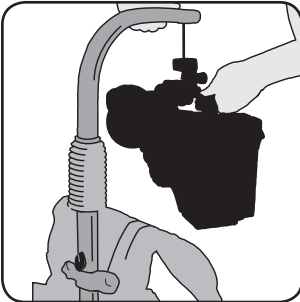
Fig. 3 Hook the camera onto the camera hook. If the camera is falling down, turn the knob for more power.
