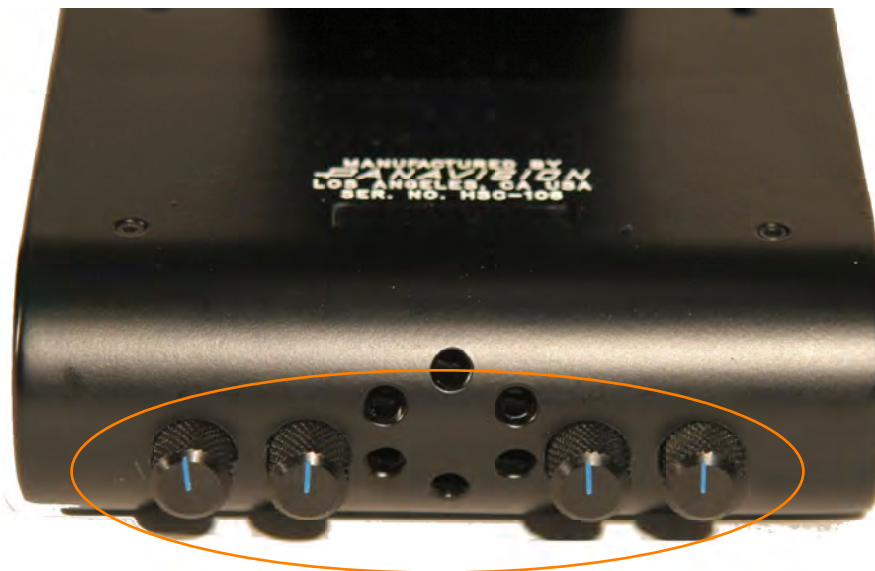
Axis Calibration knobs on controller X - Y - Z - R
