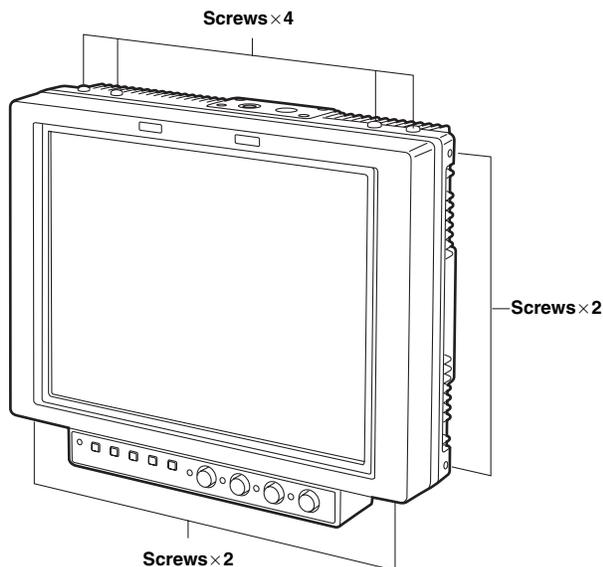
A total of eight cosmetic screws are provided with the monitor for use at such times when the main controls have been relocated. (Refer to page 8)
