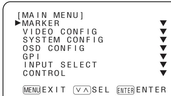
This display appears when the MENU/EXIT button is pressed. If no further action is taken for the next 120 seconds, the display will be automatically cleared.
