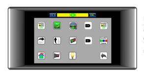
From the main menu, select Tools icon then activate Virtual Horizon When you see the horizontal bar on the top of the monitor screen, tap on CAL button. The green bubble indicates that your monitor is on level.
