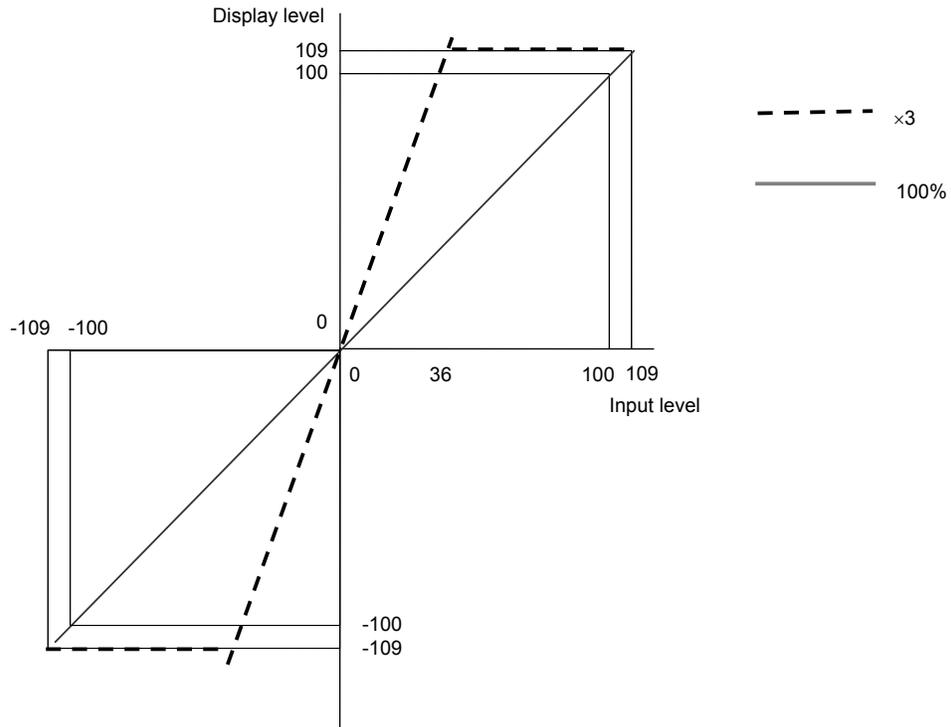
For GBR input signals, the chroma boost function works as a function for changing the B and R gain.
