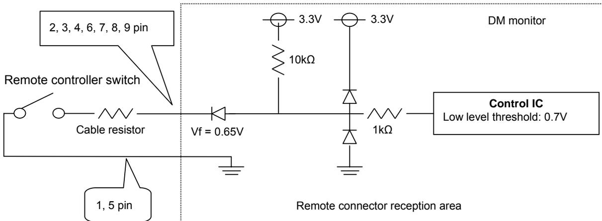
\* Design the circuitry in such a way that the cable resistance is 50Ω or less.
