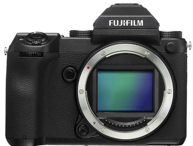
FUJIFILM GFX 50S Medium Format Camera 43.8 x 32.9 mm sensor
