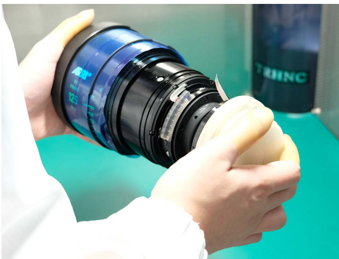
Calibrating LDS-2 lens metadata on prototypes.
