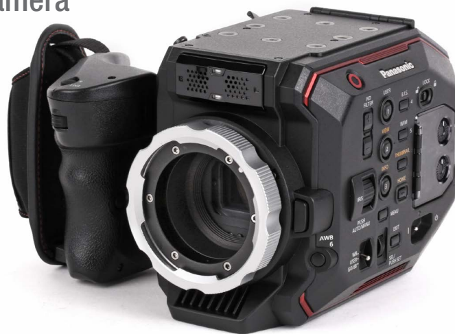
Panasonic AU-EVA1 with Wooden Camera PL Mount Conversion
