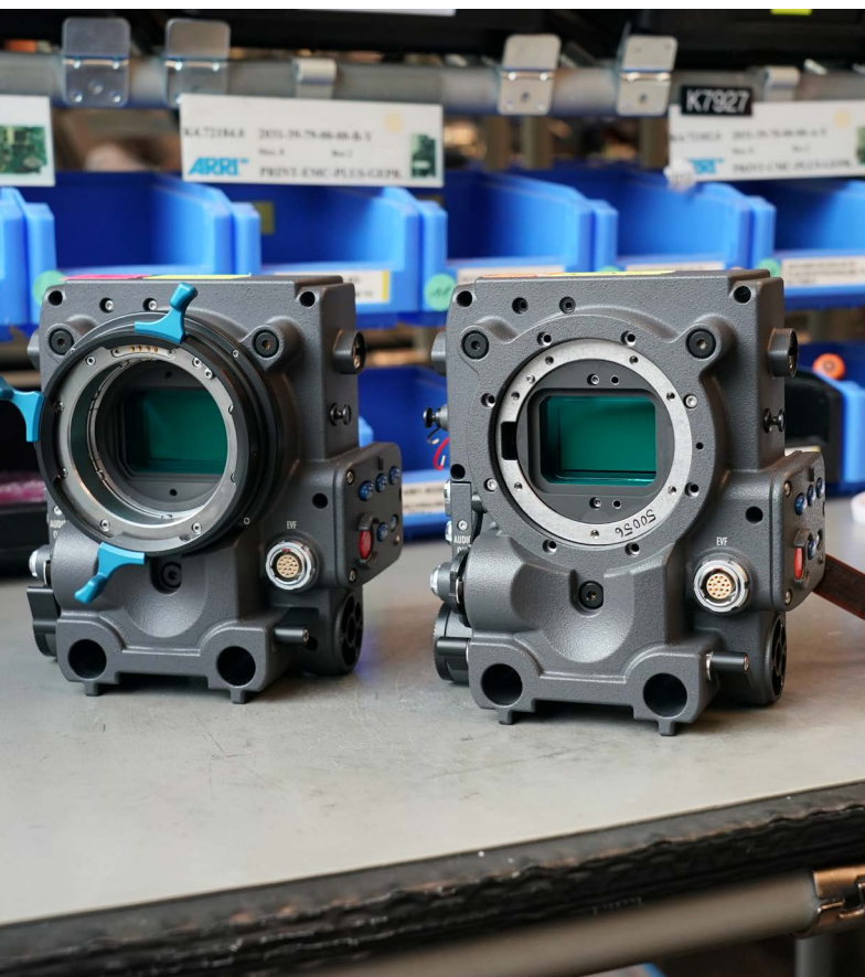
Sensor assemblies installed. Attach LPL mount to camera body on left.
