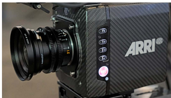
Leica M0.8 21mm f/1.4 on ALEXA Mini fitted with Leica M mount
