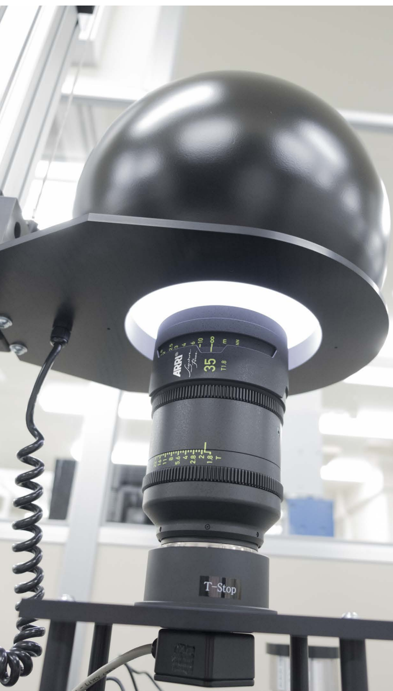
T-Stop tester ensures consistent and correct aperture values.
