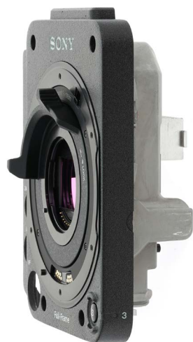
Sensor Block with Native E-mount
