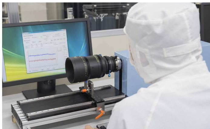
Measuring torque (lens barrel tension) for smooth operation.
