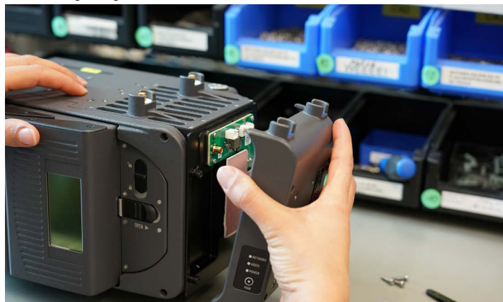
Wireless video module goes on the back.
