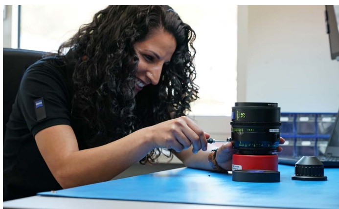
Servicing the Supreme Prime's eXtended Data connector.
