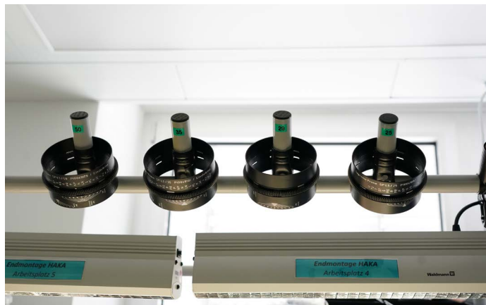
A test focus scale is selected for each focal length.
