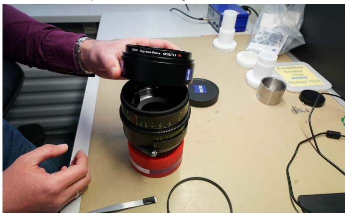
Simon removes the front assembly with front element.
