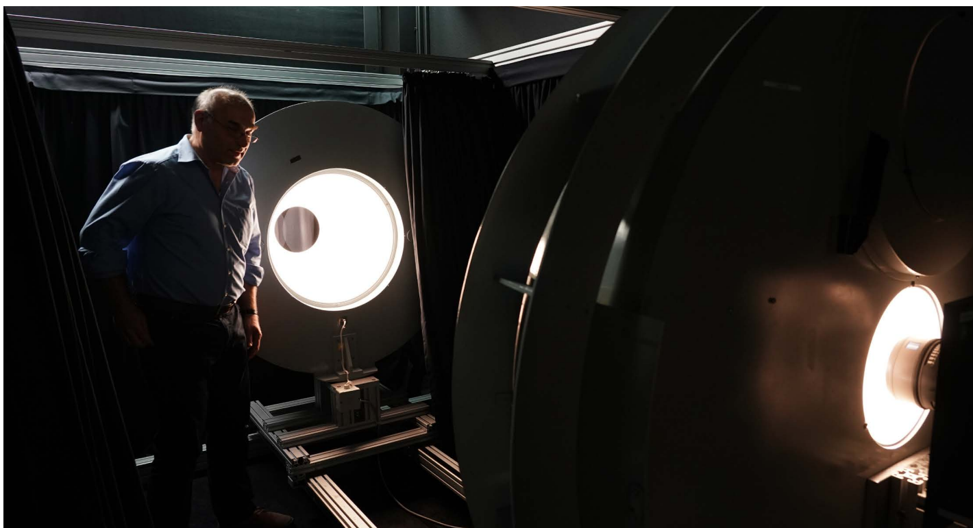
Gebhard Müller, Manager of the test lab at ZEISS checking lens performance and contrast with a “black hole” device.
