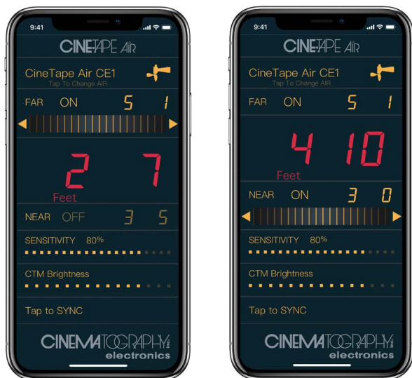
CineTape AIR App. iPhone at right shows NEAR limit ON.
