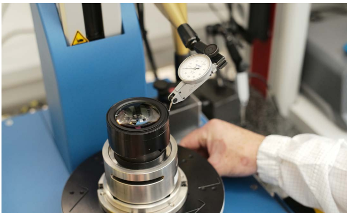
TRIOPTICS OptiCentric measures tilt and distances between individual elements—the air gaps between every lens element.
