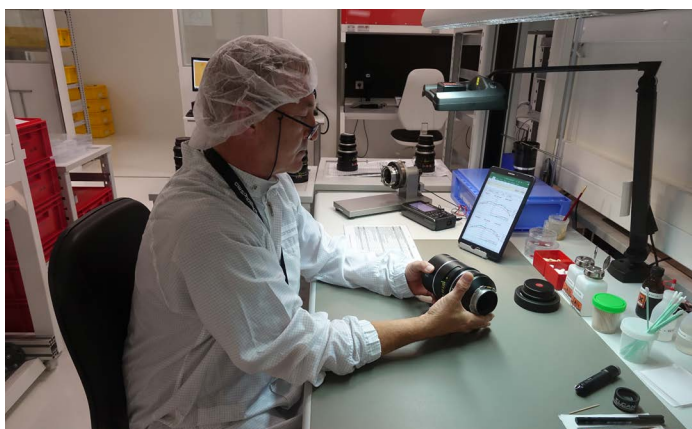
Paper creates dust as the fibers wear off. So tablets are used in the clean room for instructions, notes and communication.
