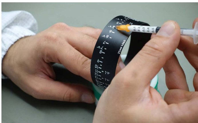
Painting the engraved focus barrel.
