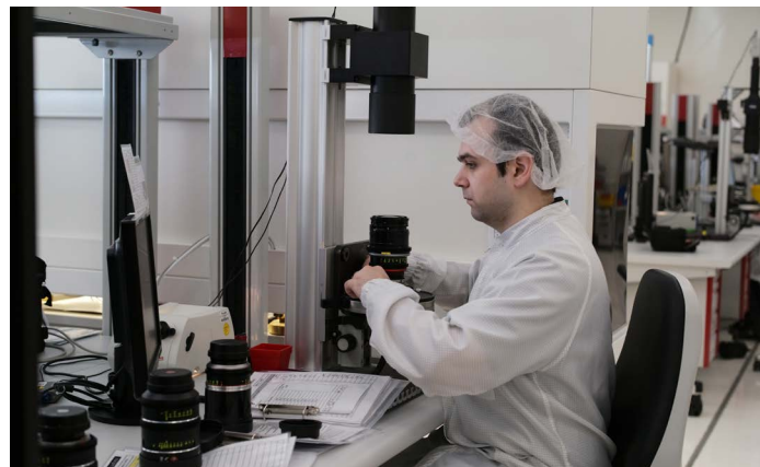
Centering and lens group adjustment on Star Test machine.
