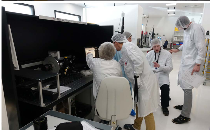
MTF Master: tests MTF curves, resolution, symmetry and performance.
