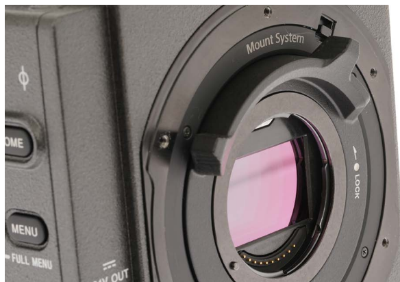
E-mount is now functional after removing the VENICE PL mount.
