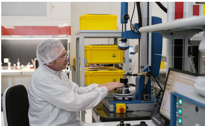
TRIOPTICS OptiCentric measures tilt and distances between individual elements—the air gaps between every lens element.
