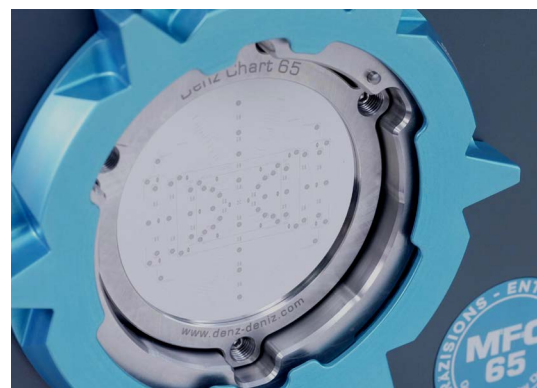
Reticle with spherical and anamorphic Siemens stars, line pairs blocks, frame lines and image circles.
