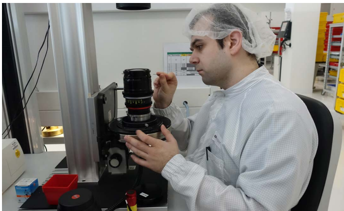
Air gap in a Summilux-C can be 1/10mm, with 1/100mm tolerance.
