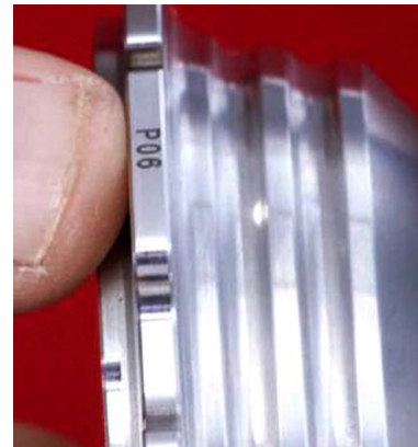
Offset code for tolerance compensation.
