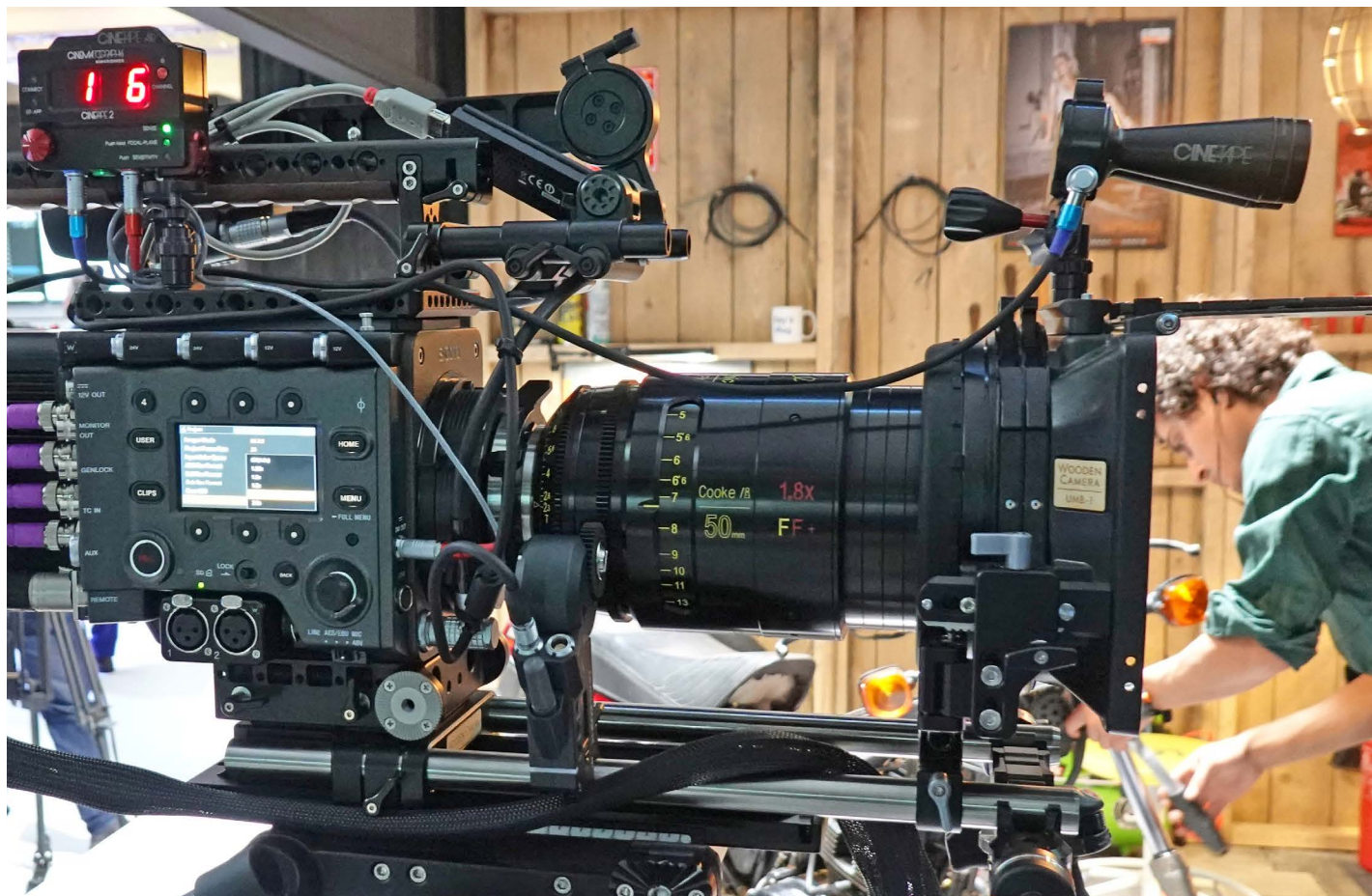
ARRI, RED and Sony have implemented 1.8x desqueeze. Above: Cooke 1.8x Anamorphic /i T2.3 Full Frame Plus on Sony VENICE with CineTape2. Below, Larry Barton, President of Cinematography Electronics setting up new CineTape2 on Sony VENICE.
