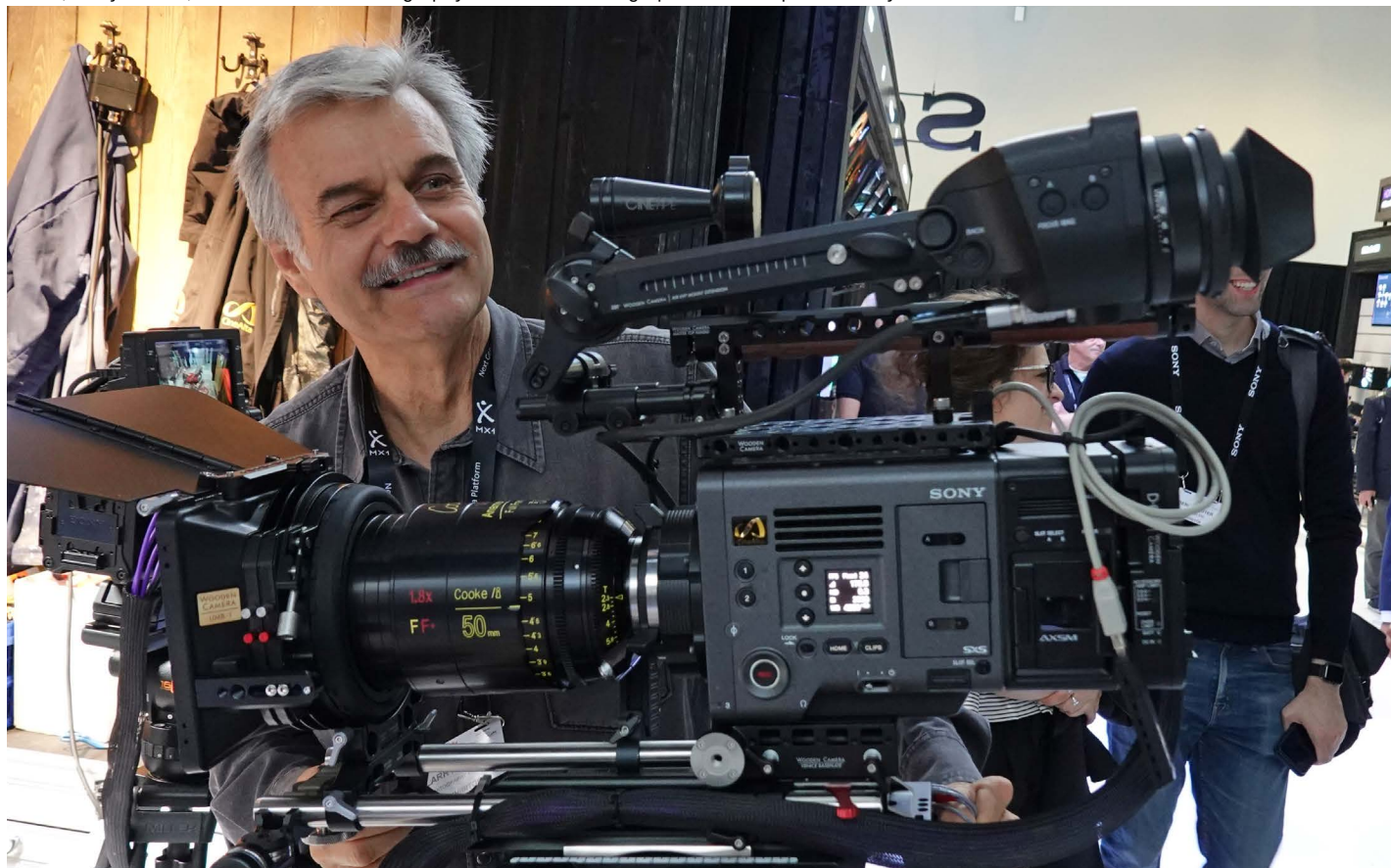
ARRI, RED and Sony have implemented 1.8x desqueeze. Above: Cooke 1.8x Anamorphic /i T2.3 Full Frame Plus on Sony VENICE with CineTape2. Below, Larry Barton, President of Cinematography Electronics setting up new CineTape2 on Sony VENICE.
