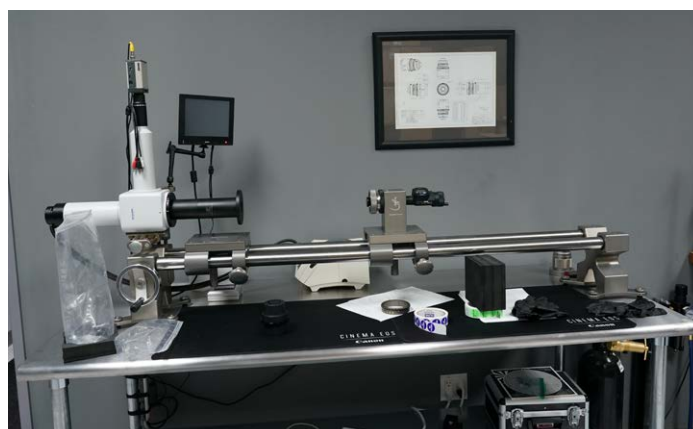
Gecko collimator in the lens test room.
