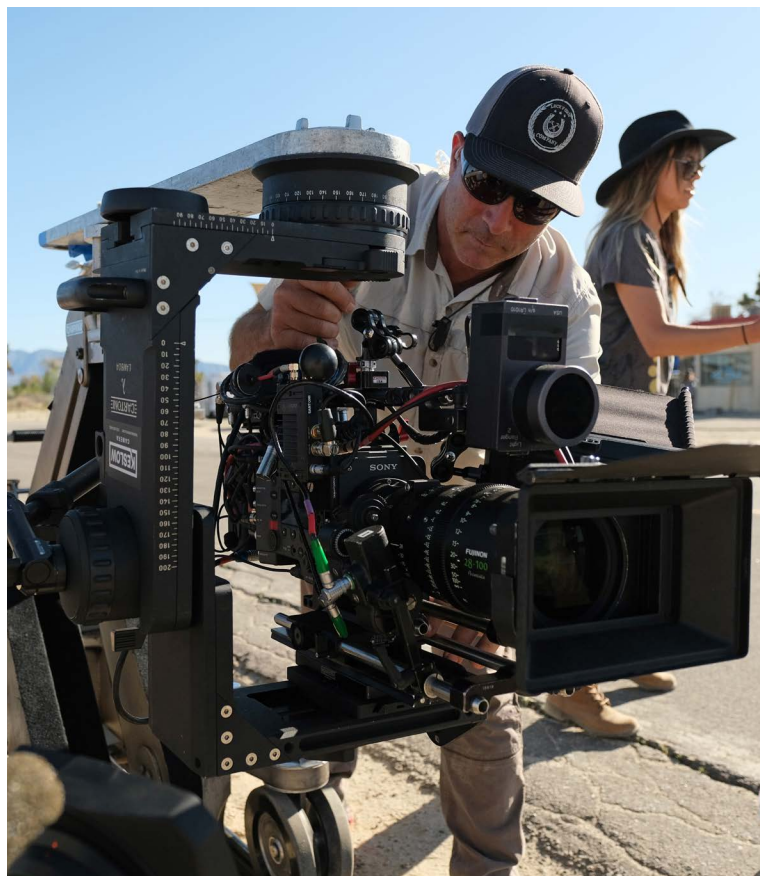
Underslung Cartoni Lambda Head, Premista, Light Ranger 2...
