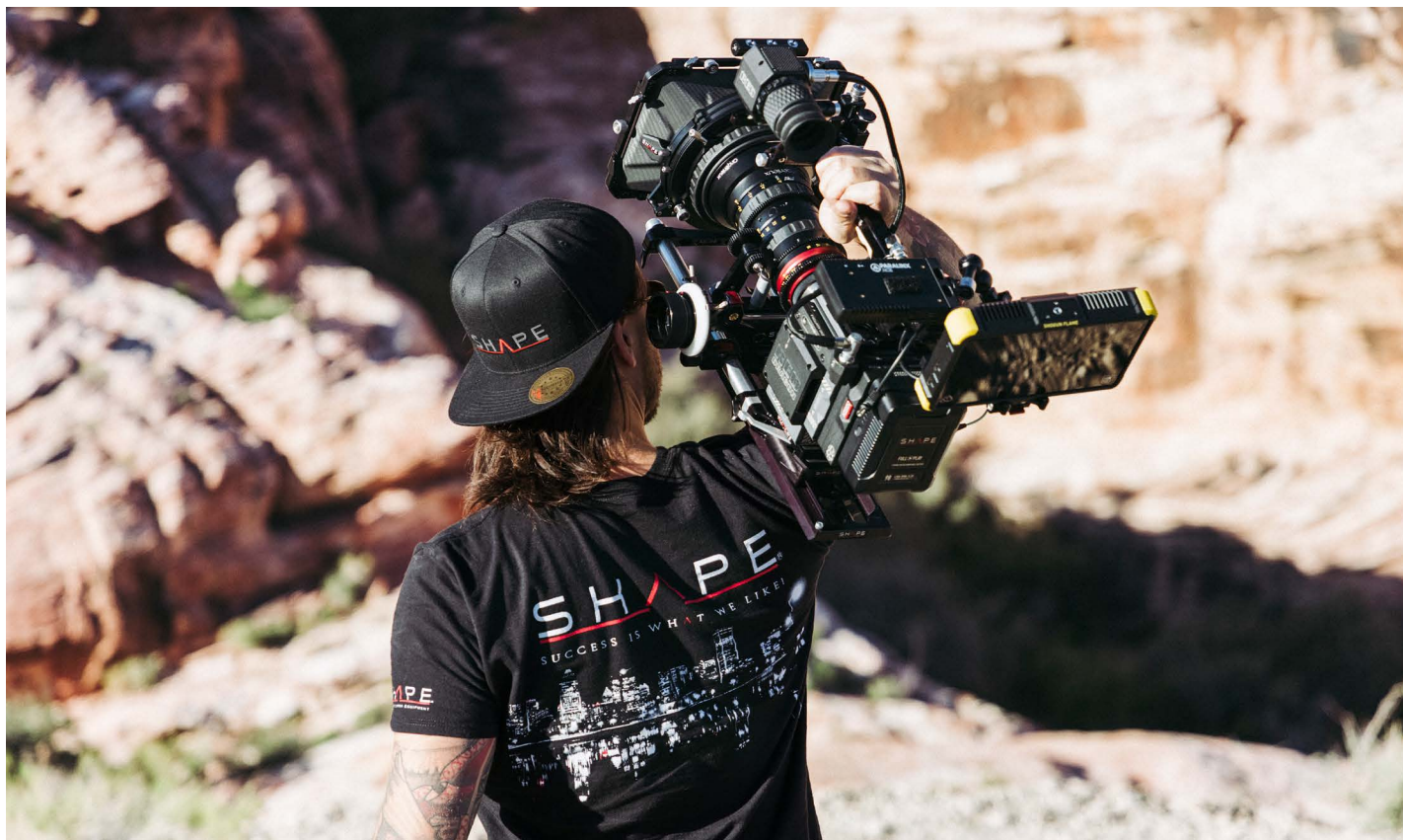
Mylène Girard et Charles Vallières, above, owners and founders of SHAPE WLB, in Nevada's Valley of Fire prior to NAB 2019 with SHAPE's fully rigged and ready RED system. From front to back: SHAPE mattebox, support, follow focus, handle, eyepiece support, SHAPE Full Play battery and brackets. @SHAPEwlb #SHAPetheworld #SHAPEshooter
