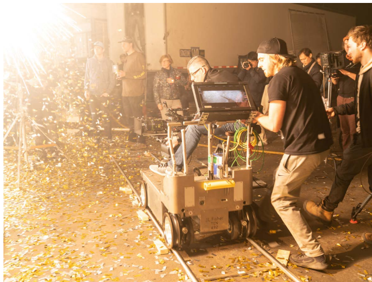
Dollying through the pyrotechnics on Fisher 10 with TTWs (Track Tires).
