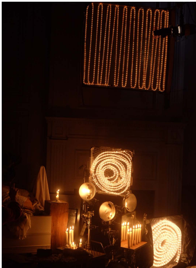
Rope light. "We created frames of different sizes with these garlands. They allowed us to combine the brightness of small bulbs and to be able to work with fairly large sources." — Claire Mathon, AFC.
