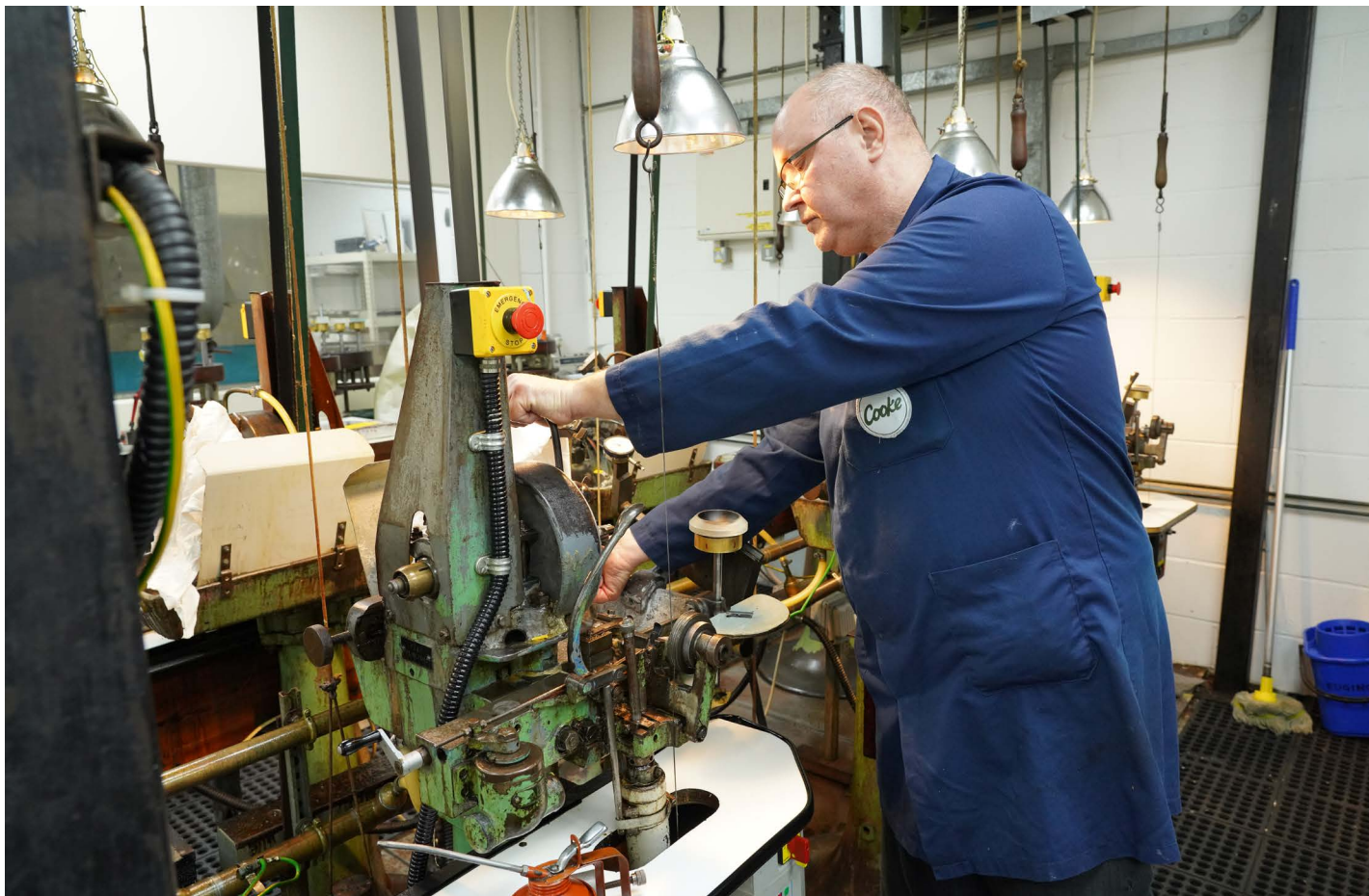
Vintage machines in the hands of a master craftsman like Paul Utting can produce accurate results to tolerances of less than 5 microns.
