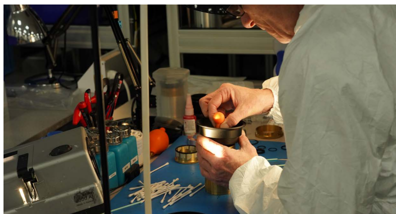
The precise edging done earlier pays off as lenses mount inside barrels.
