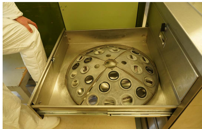
Load the optical elements onto carrier.
