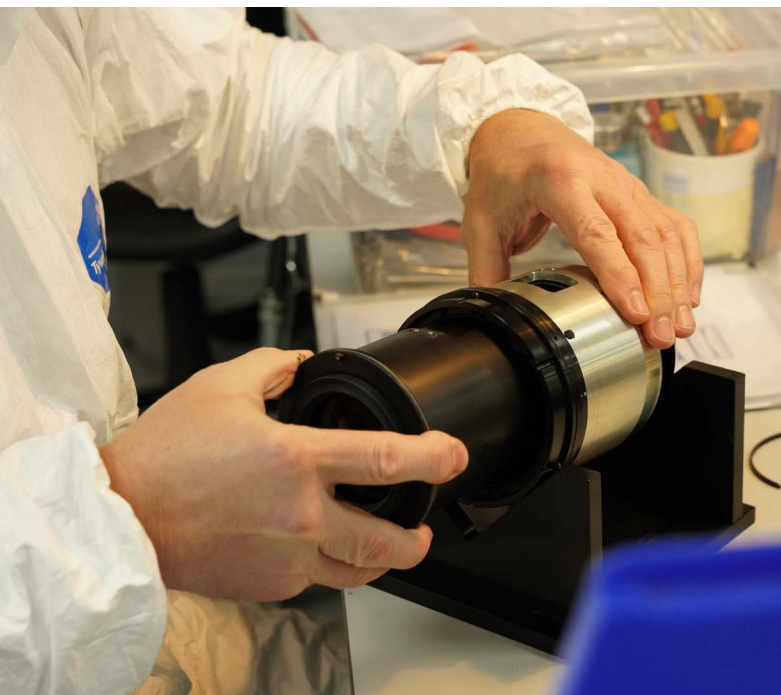
Inners (sub assemblies) slide into outers, below.
