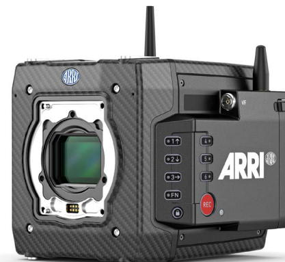
ALEXA Mini LF with lens mount removed
