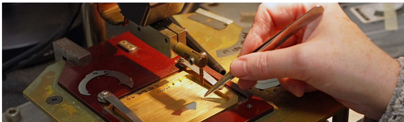
Iris leaf pins are welded into position.
