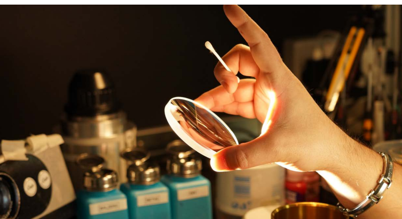
Lens elements are cleaned and inspected again.
