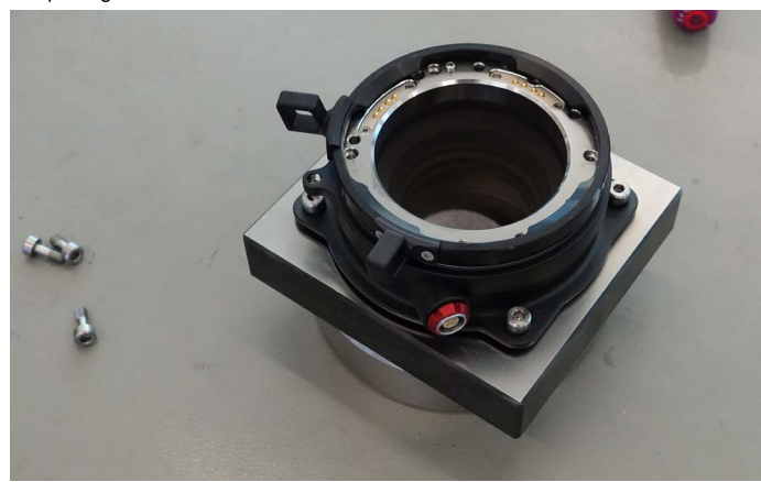
PL mount for AMIRA and MINI cameras with LDS and /i data contacts
