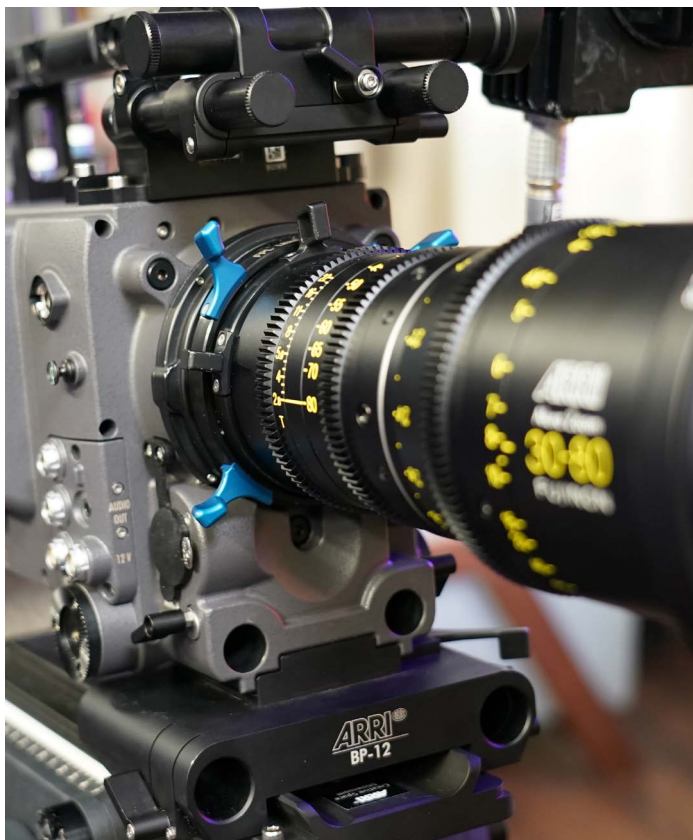
PL-to-LPL adapter accepts any PL mount lens on ALEXA LF. The PL mount has 2 traditional black ears. The LPL mount has 3 blue ears.
