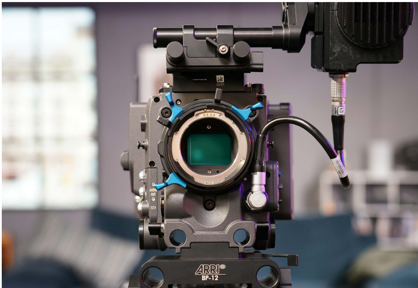
PL-to-LPL adapter accepts any PL mount lens on ALEXA LF. The PL mount has 2 traditional black ears. The LPL mount has 3 blue ears.
