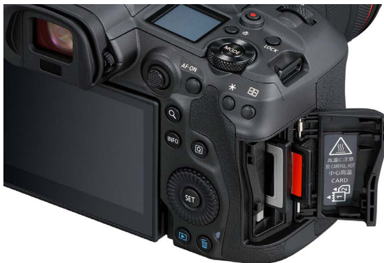
R5 has one slot for CFexpress card and another slot for an SD UHS-II.
