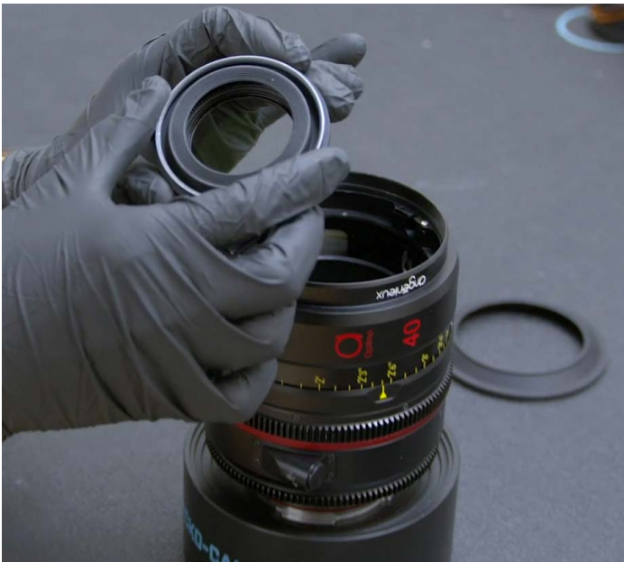
Above: Removing Angénieux Optimo Prime's Internal Optical Element in Band Pro Clean Room.
