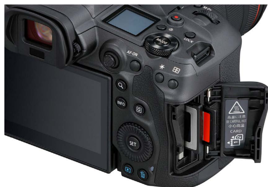
R5 has one slot for CFexpress card and another slot for an SD UHS-II.
