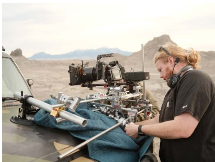
DJI Ronin 2 as remote head controlled from inside car. The Ronin 2 also worked as a handheld gimbal, along with a DJI FPV, and Mavic 3.
