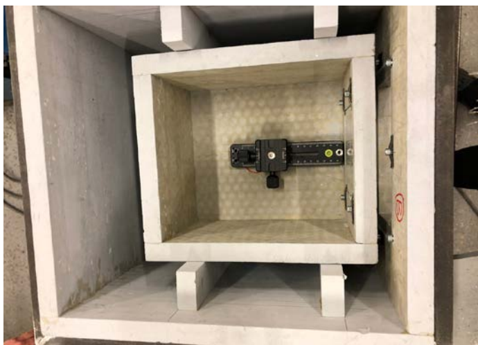
Fireproof box with silicate walls for Blackmagic Micro camera.
