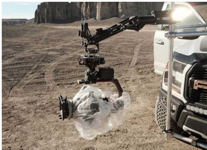
DJI Ronin 2 as remote head controlled from inside car. The Ronin 2 also worked as a handheld gimbal, along with a DJI FPV, and Mavic 3.
