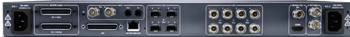
Ethernet and Fiber Inputs and Outputs
