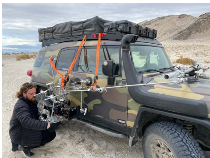
DJI Ronin 2 as remote head controlled from inside car. The Ronin 2 also worked as a handheld gimbal, along with a DJI FPV, and Mavic 3.
