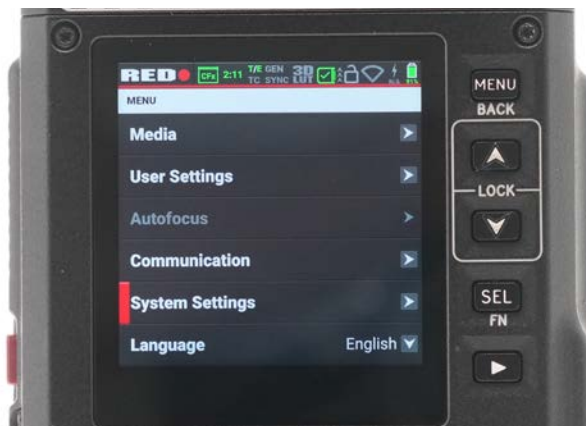
2. Push Menu button to go to home page. Navigate with Up and Down arrow keys and SEL to Select. Let's select System Settings.
