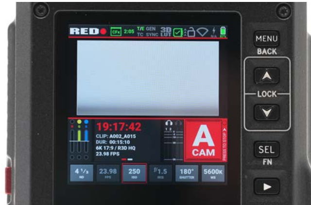
6. Here, we see 4 1/3 stops of light reduction. Because it is continuously variable, showing stops is easier than wondering if it's ND1.3 or ND1.4.
