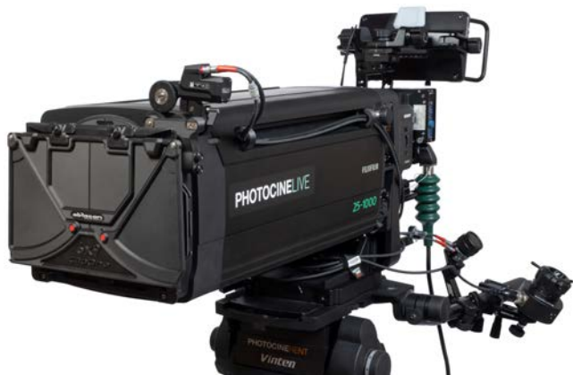
The top eyebrow and side flaps fold in to cover the front of the lens.
