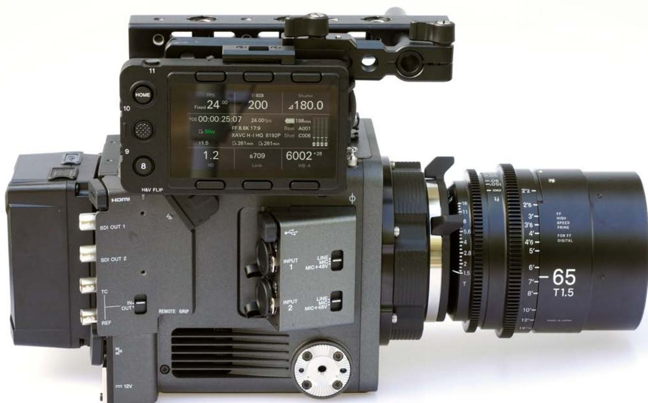
Attach the EVF Monitor on the camera right side for a VENICE style menu main display
