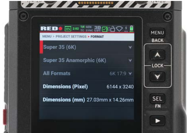
10. Format, Resolution, Aspect Ratio and sensor dimensions helpfully appear.
