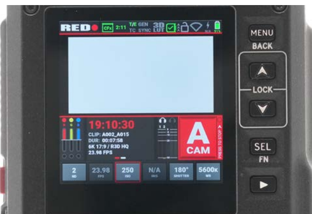
5. Seeing actual stops of light lost is nice—less math on set. Adjust ND, fps, ISO, iris, shutter and white balance directly on touch screen.
