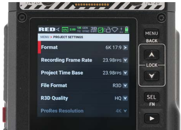
12. Recording fps (in-camera); Project Time Base (fps at which images will be viewed); File Format for REDCODE RAW or ProRes; and Quality.
